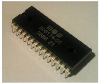
Fig. 1 - Source c64-wiki.com failures: the PLA chip, codenamed MOS 906114-01.
