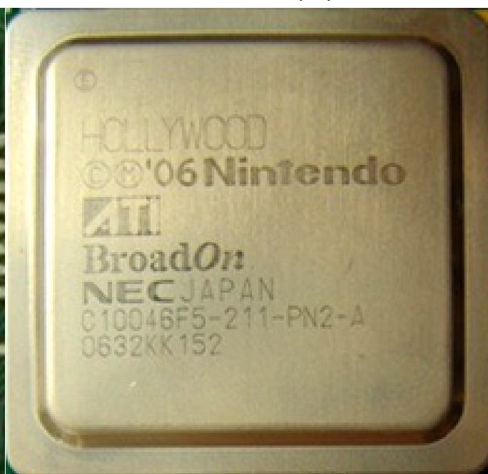
On the one hand the IBM Broadway CPU at its side the ATI Hollywood GPU.
