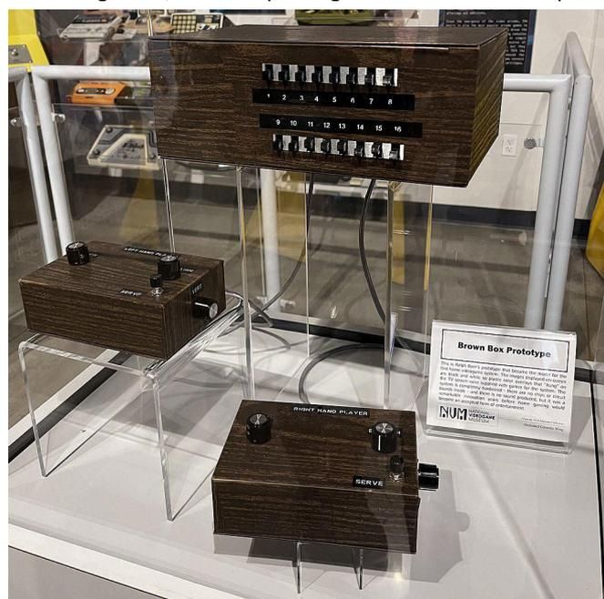
**Fig. 3 - a prototype of the Brown Box, so called because of the brown scotch tape used to simulate the grain of the wood**
