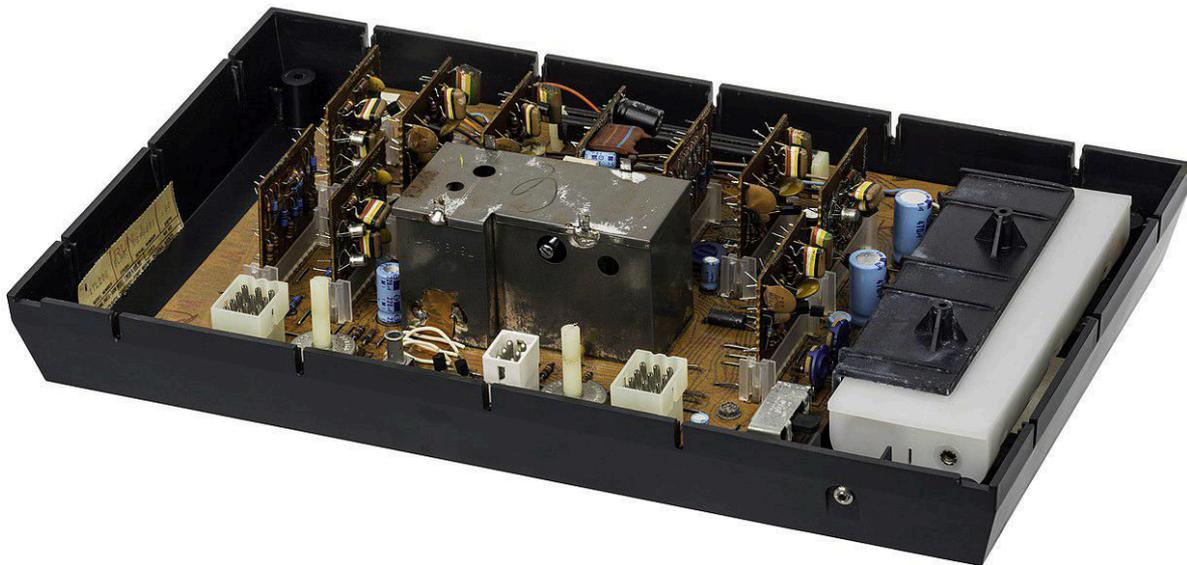
**Fig. 4 - Interior of the Odyssey. You can see the circuits made with discrete components (photo: Evan-Amos)**
