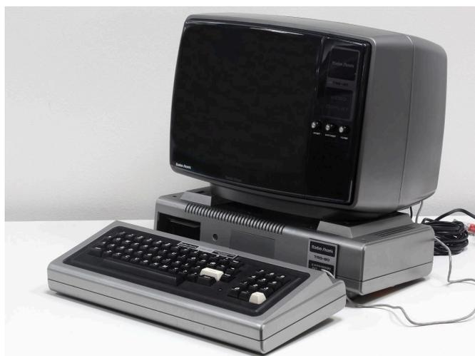
**Fig. 5 - A TRS-80 Level II with the Expansion Interface**
