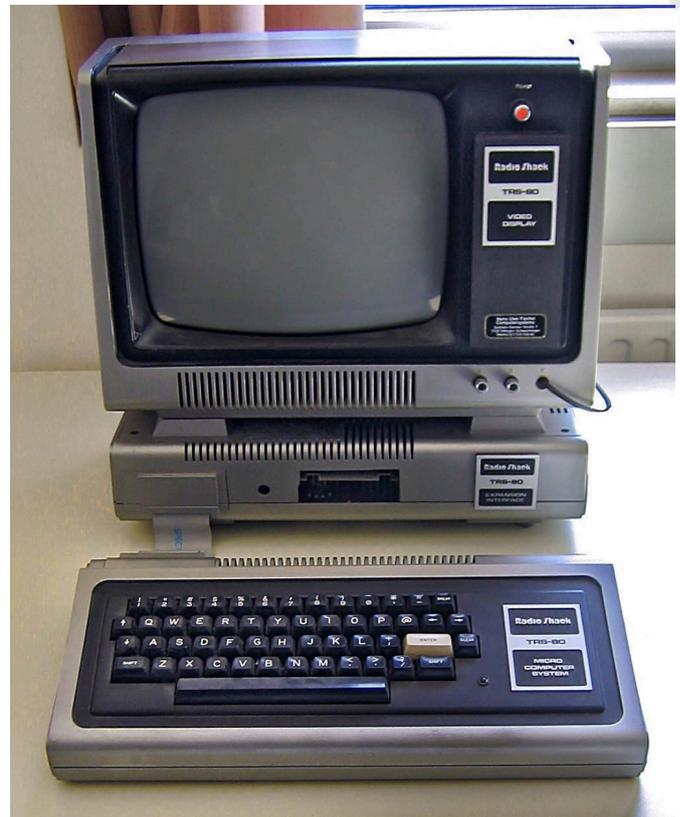
**Fig.4 - A TRS-80 Level I (note the keyboard without the numeric keypad) with Expansion Interface (the additional case placed under the monitor) (photo by Flominator, source Wikimedia Commons)**
