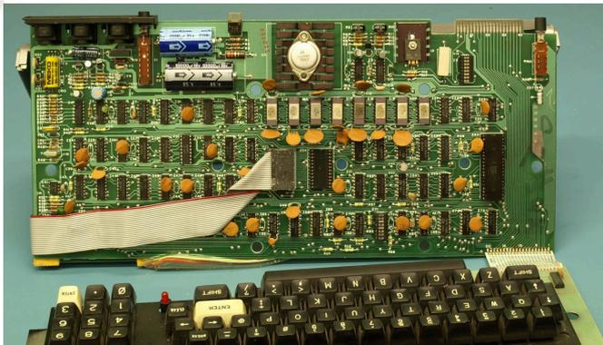
**Fig. 2 - The motherboard of the first version of the TRS-80 - the large chip on the right is the Zilog Z80 (photo by Binarysequence, source Wikimedia Commons)**
