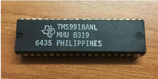
Figure 2: TMS9918A Video Display Processor
