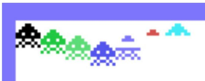
Figure 1 - TMS9918 displays only 4 sprites per scan line
